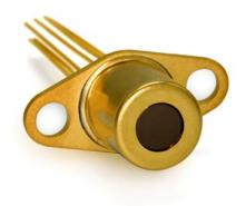
The device has minimum responsivity of  $1.2 \times 10^5$  V/W with the active-element temperature controlled to -30 °C. Housed in a standard TO37 can, the unit has a 2 mm² active area. Absolute ratings for storage and operating temperatures range from -40 °C to +85 °C. Additional uses include carbon monoxide gas analysis, environmental monitoring, process control systems, and industrial burner monitoring and control.
